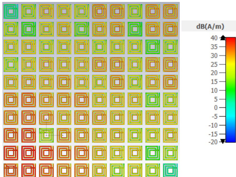
Figure 4.16 – Current density obtained by simulation using CST ® for the 10 \times 10 cells MCWPT system operating at f = 13.56 MHz. The colors represent the density of the current obtained with the simulation.
